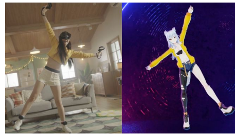
Figure 1. An illustration depicting the operation of full-body tracking systems in VR. The left side shows a person wearing an HMD, holding controllers, and equipped with body trackers on the belt and legs. On the right side, the person's digital body is visible, with its movements synchronized with the physical body movements through tracking systems. The person sees their digital body through the HMD from a first-person perspective, aligned with the position of their physical body. Source
